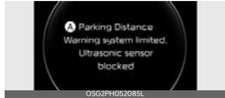
A: Parking Distance Warning system limited. Ultrasonic sensor blocked
