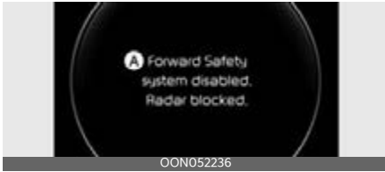
A: Forward Safety system disabled. Radar blocked
