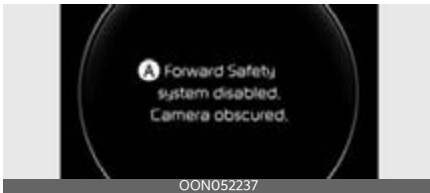
A: Forward Safety systems disabled. Camera obscured
