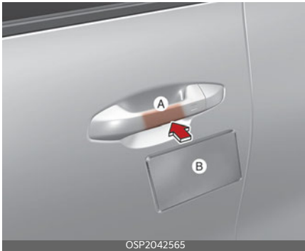
[A]: Door handle authentication pad, [B]: Card key NFC antenna
