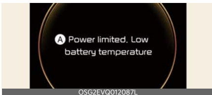
A: Power limited. Low battery temperature
